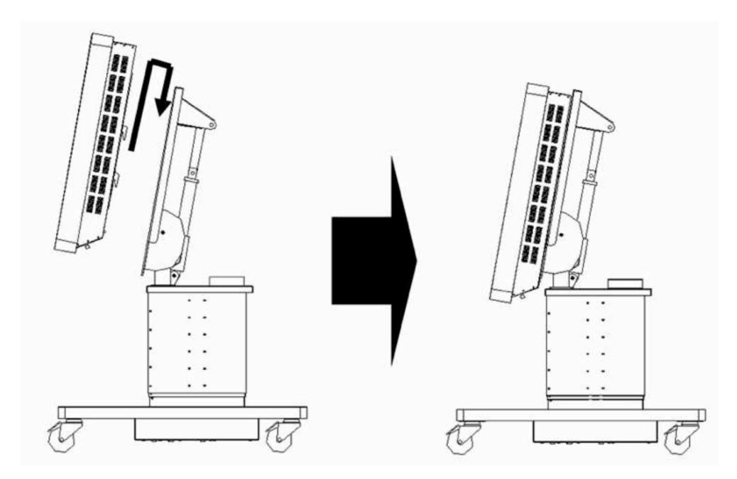
3-1-4. Secure the LCD in position with the 6 fastening bolts (M6\*L10mm), see hole locations on the diagram below.
