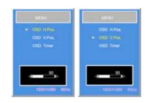
Press "enter" and " $\blacktriangle$ " or " $\nabla$ " to select, and to move the OSD position in horizontal, or, vertical direction.
